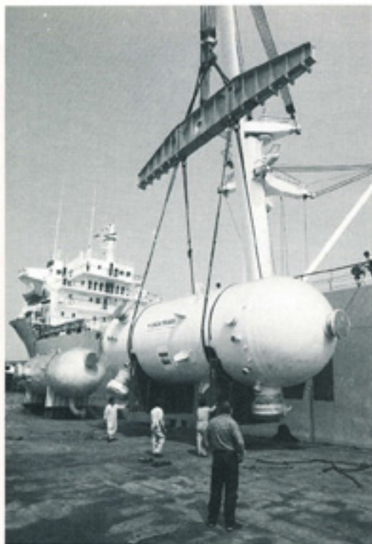
The m.s. "Project Orient" loaded 2 production separators and 2 condensate water stripping columns in the port of Rotterdam with weights ranging from 114 to 157 tonnes. They were destined for Ulsan in Korea to be part of the Goodwin "A" project.
